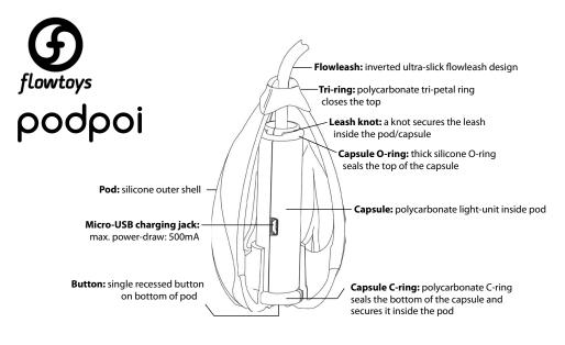
Length: 118mm | Diameter: 66mm | Weight: 128g | Battery: 3.7v, 750 mAh rechargeable Li-ion
