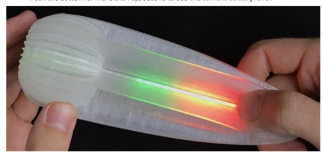
After 10 minutes of inaction in menu mode, the poi automatically turns itself off.
