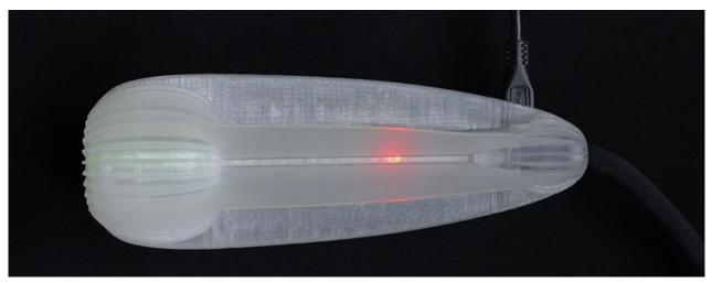
When the poi is on charge, the red light slowly moves towards the end of the poi. When the poi is completely charged, the light finally turns green.
